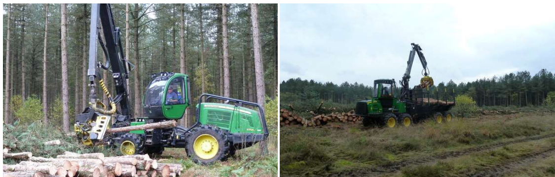
Figure 5: Pictures showing a harvester (left) processing harvested roundwood into assortments, and a forwarder (right) loading roundwood (source: Ecopedia, n.d.).
