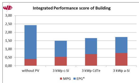
**Figure 4:** Integrated score of life-cycle environmental impacts combining the MPG material score and a weighted energy consumption indicator (EPG\*).
