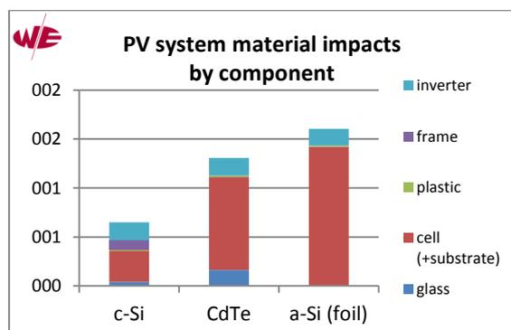
**Figure 6:** Contribution of PV system components to aggregated impact scores. Note that for a-Si foil the stainless steel foil has been included in the cell material.
