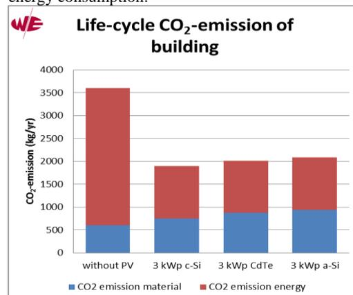
**Figure 3:** Life cycle CO<sub>2,eq</sub> emissions from building with different PV installations.
