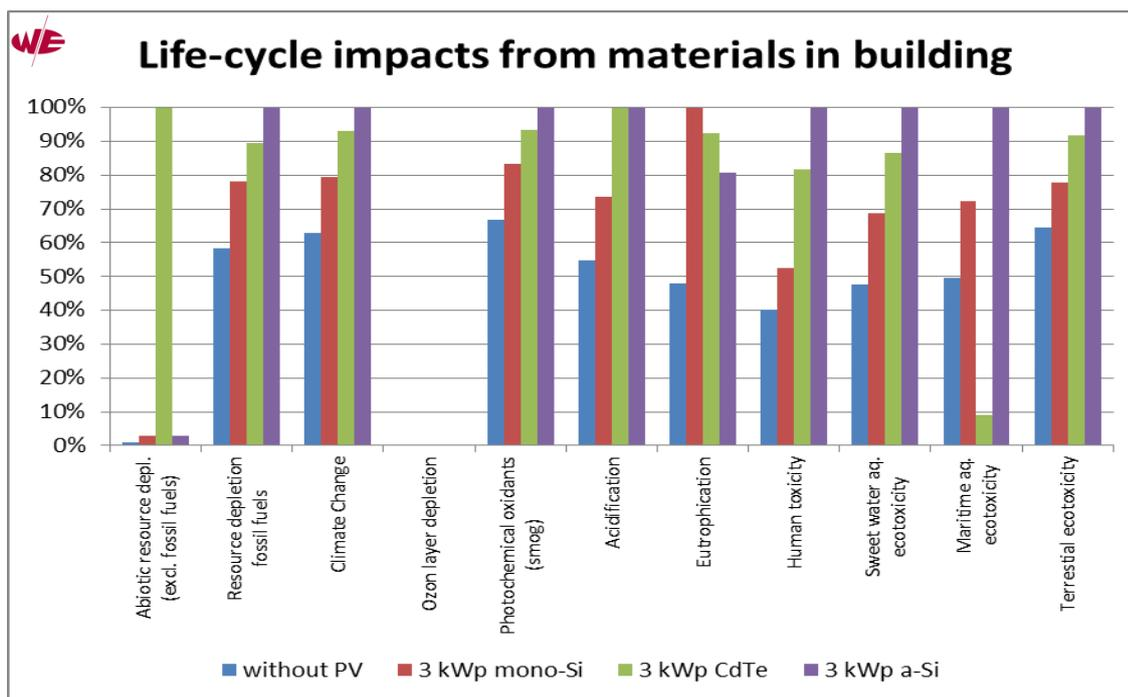
**Figure 5:** Characterized life cycle impacts from semidetached house with 3 kWp PV system, employing different PV technologies.
