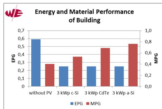
**Figure 2:** Materials impact score (MPG) and Energy Performance Score (EPG) of a house with different PV installations. N.B. EPG and MPG scores have different units.
